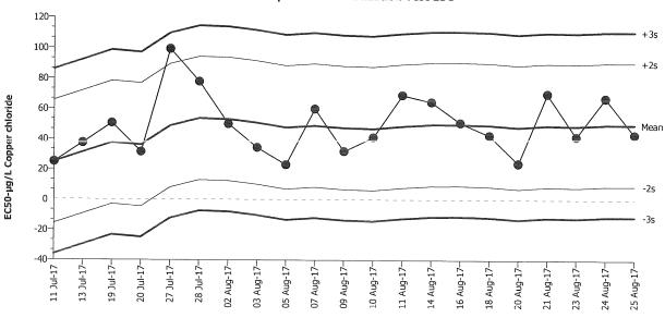
Mean: 49.6 Count: 20 -2s Warning Limit: 8.924 -3s Action Limit: -11.42 Sigma: 20.34 CV: 41.00% +2s Warning Limit: 90.28 +3s Action Limit: 110.6
